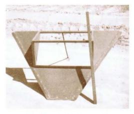
The Portable Weir is a precision water measuring device for all standard concrete ditches. This Weir is patterned after an old proven system used by the Salt River Project and the Roosevelt Water Conservation District of Arizona for over 50 years.
