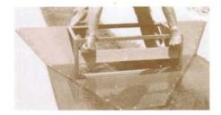
7. When the Weir has no air pocket at the crest, it is called a Submerged Weir. The measuring stick provided with the Weir can only be used with the free falling Weir. In an instance like this a measurement can be taken with the use of the Clausen water rule which has a piezometer tube that will measure the difference between the upstream head and the downstream head. In most all instances the measuring stick provided will be able to make measurements.
