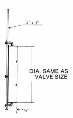
The Clip Type Valve is designed for use in concrete lined ditches, where a simple flow control valve is suitable. Clip valves are readily available for an 8", 12" or 14" port, or can be specially ordered in larger sizes. Rings, lids or handles can be ordered separately.
